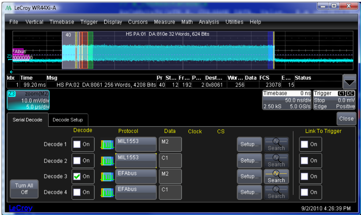
Figure 1: The Serial Decode Dialog is the entry point to the Decoders. It allows the setting of the sources as well as turning the Decoders on and off.
