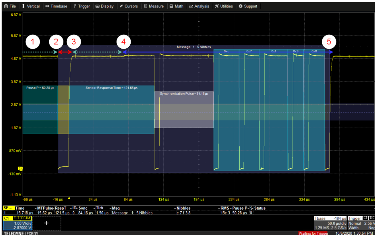
Figure 2: Triggering from master and answer by a slave with a digital push-pull output driver
