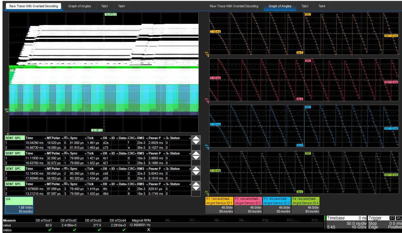
Figure 10 Measurement on 4 identical sensors, 1 and 3 shifted by 180 degrees, with magnet at 12.85 rps
