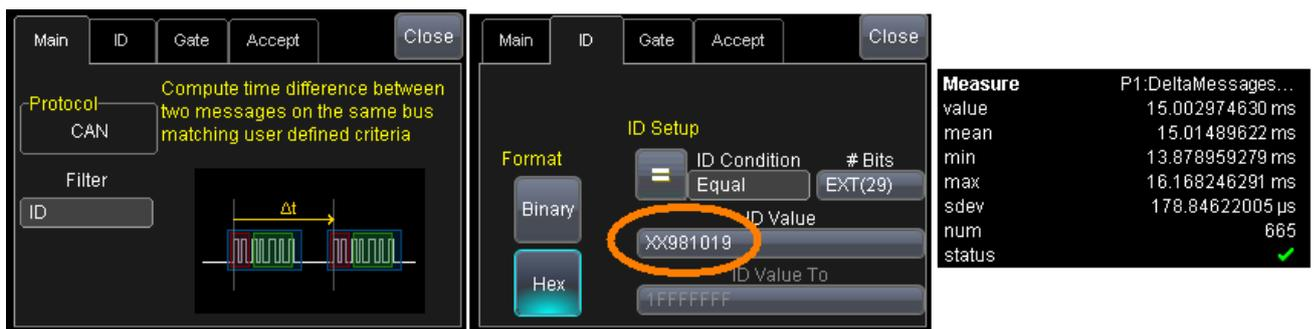
Figure 5: The DeltaMessage Parameter settings (left) and results (right) for monitoring CAN ID 0x981019 on the bus, shows a mean distance of 15.01 [ms].
