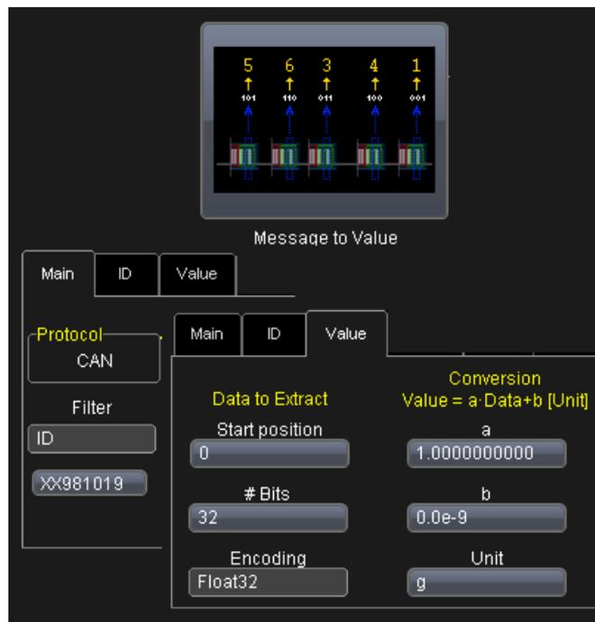
Figure 7: Setup of the MessageToValue parameter for the X acceleration, a 32 bit subfield of message 0x981019, located at bit 0. (See also Fig. 3)
