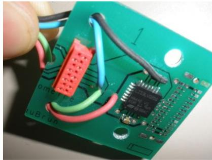
Figure 2: The LIS3LV02DQ inertial sensor mounted on a small PCB is the heart of the acquisition system, and delivers the necessary data to assess passenger's comfort in real time.
