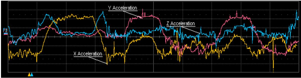
Figure 8: This is the normal 3D output of the LIS3LV02DQ inertial sensor when manipulated softly. Accelerations remain between  $\pm 1$  [g] in all directions.
