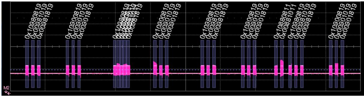
Figure 4: Snapshot of the overall CAN traffic on the CAN bus (250 kb/s) of a moving vehicle.
