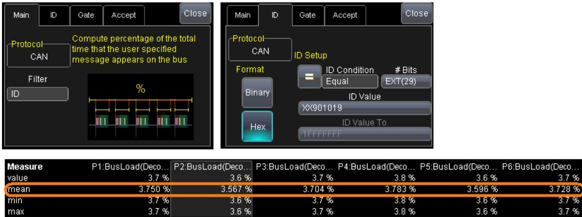
Figure 6: The BusLoad parameter, with its setting and results, used on 6 of the messages, establishes that each message uses about 3.7 % of the bus bandwidth. This correlates with the fact that a message of 500 [μs] is broadcasted every 15 [ms], therefore a busload of 3.3 %. The extra 0.4% is explained by the fact that a complete message length encompasses the CAN Inter Message Gap after the last bit.
