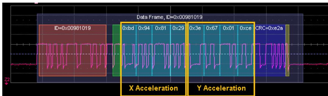
Figure 3: Typical CAN Frame 0x981019, containing X and Y accelerations expressed as IEEE754 floating point numbers. The message length is about 125 bits (with slight variations due to the insertion of the stuff bits), and spans a time of 500  $\mu$ s since every bit is 4  $\mu$ s long.
