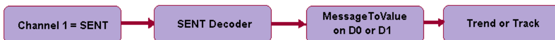
Figure 6: 3 Step processing chain of the oscilloscope, from Raw Data on the Channel to the Graph
