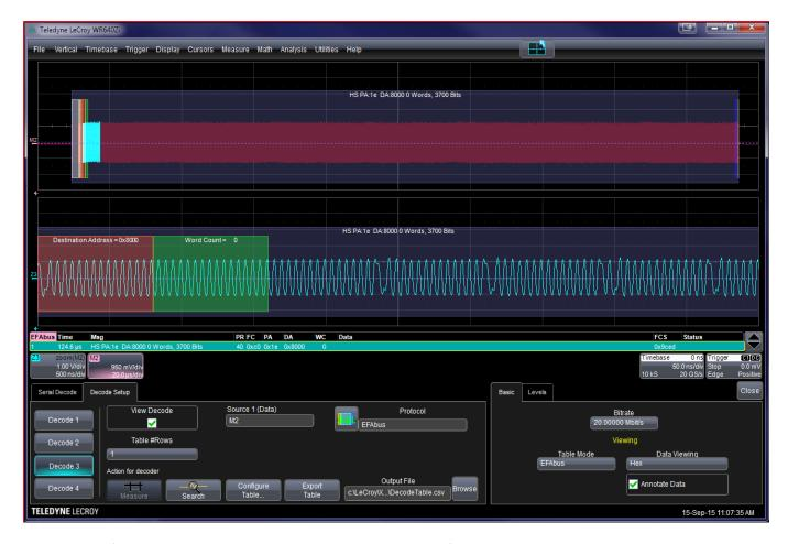
The header of the HS Frame is decoded, the CRC is decoded and found correct, but the data words are NOT decoded. The zoom shows the incorrect WC embedded of 0 causing the problem. Furthermore no error is flagged to alert the user.
