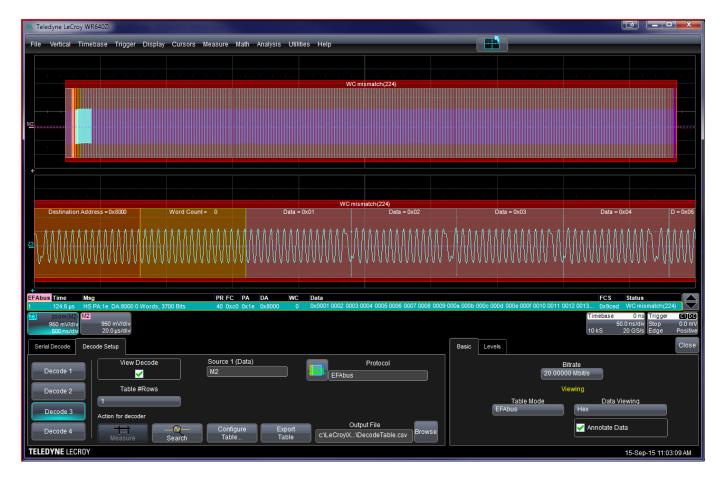
The complete Frame is now decoded, **including data words.** This is in line with the philosophy that all decoders will do their best to interpret the data, even faulty, **but** the decoder will flag errors and attempt to provide information to the engineers. This behavior helps understanding the root cause of the issue and fix it.
