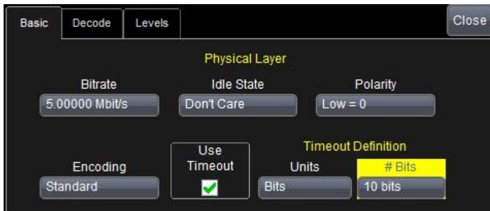
Figure 4: The 3 tabs (Basic, Decode, Levels) driving Manchester and NRZ decode.
