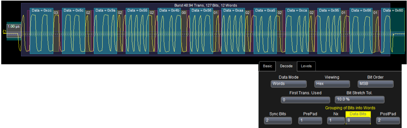
Figure 25: Payload bits grouped as repeated \langle 1 | 1x8 | 2 \rangle blocks
