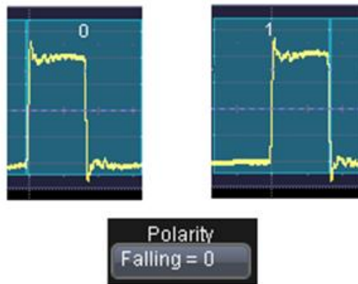
Figure 9: Manchester Physical to Logical mapping, case Falling = 0
