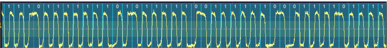
Figure 14: Differential Bi-Phase Space, always Midbit change, "0" no change at bit start and "1" changes
