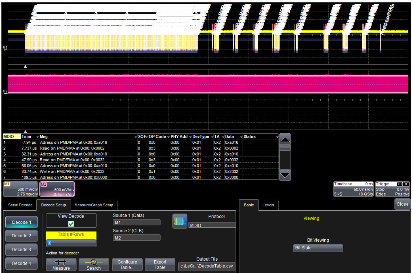
Figure 3 Initial decoding of 858 MDIO commands on 2 memory traces, M1 and M2
