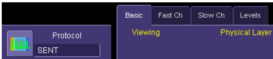
Figure 2: The protocol selection governs the appearance of the Right Hand Side tabs.
