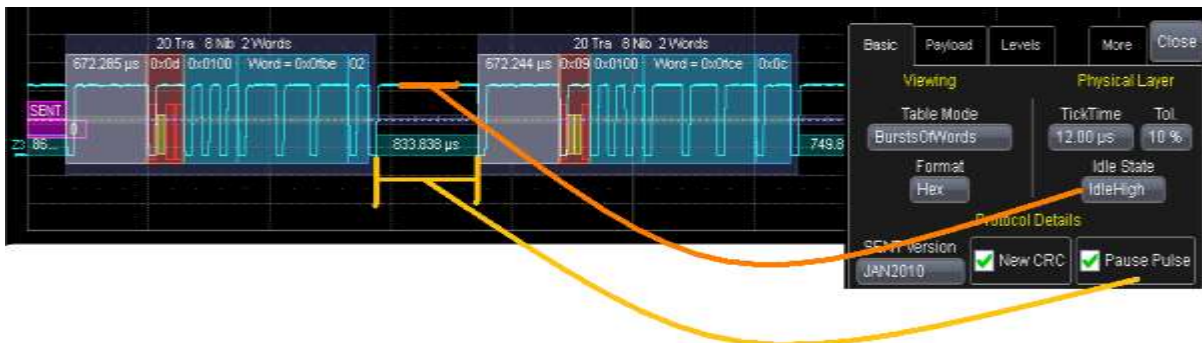
Figure 20: Example of SENT signal, 12 µs TickTime, Idle high with Pause Pulse
