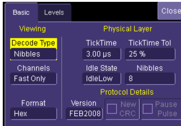
Figure 3 When Decode Type is Nibble, only the Basic and Levels tabs are required
