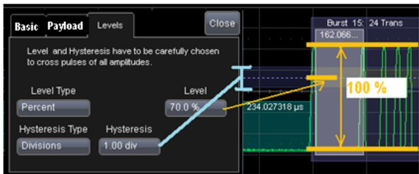
Figure 9: The Level controls and there visualization on trace
