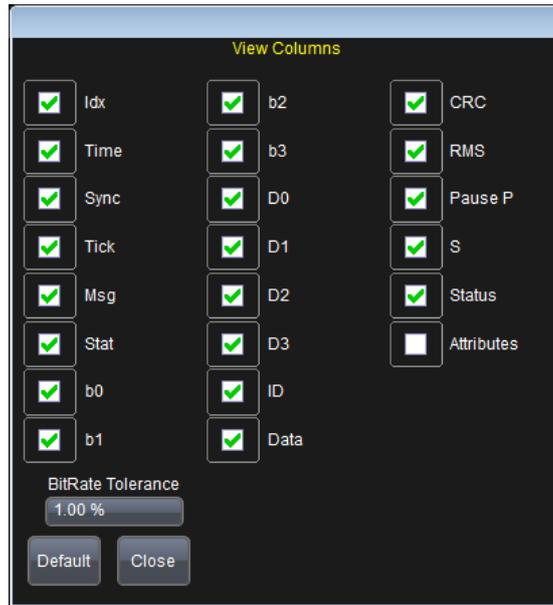
Figure 31: The columns of the SENT decoder
