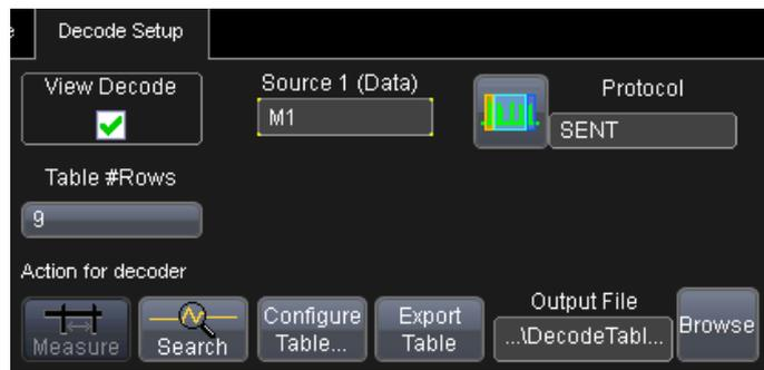
Figure 1: The selection of SENT in the Decode Setup
