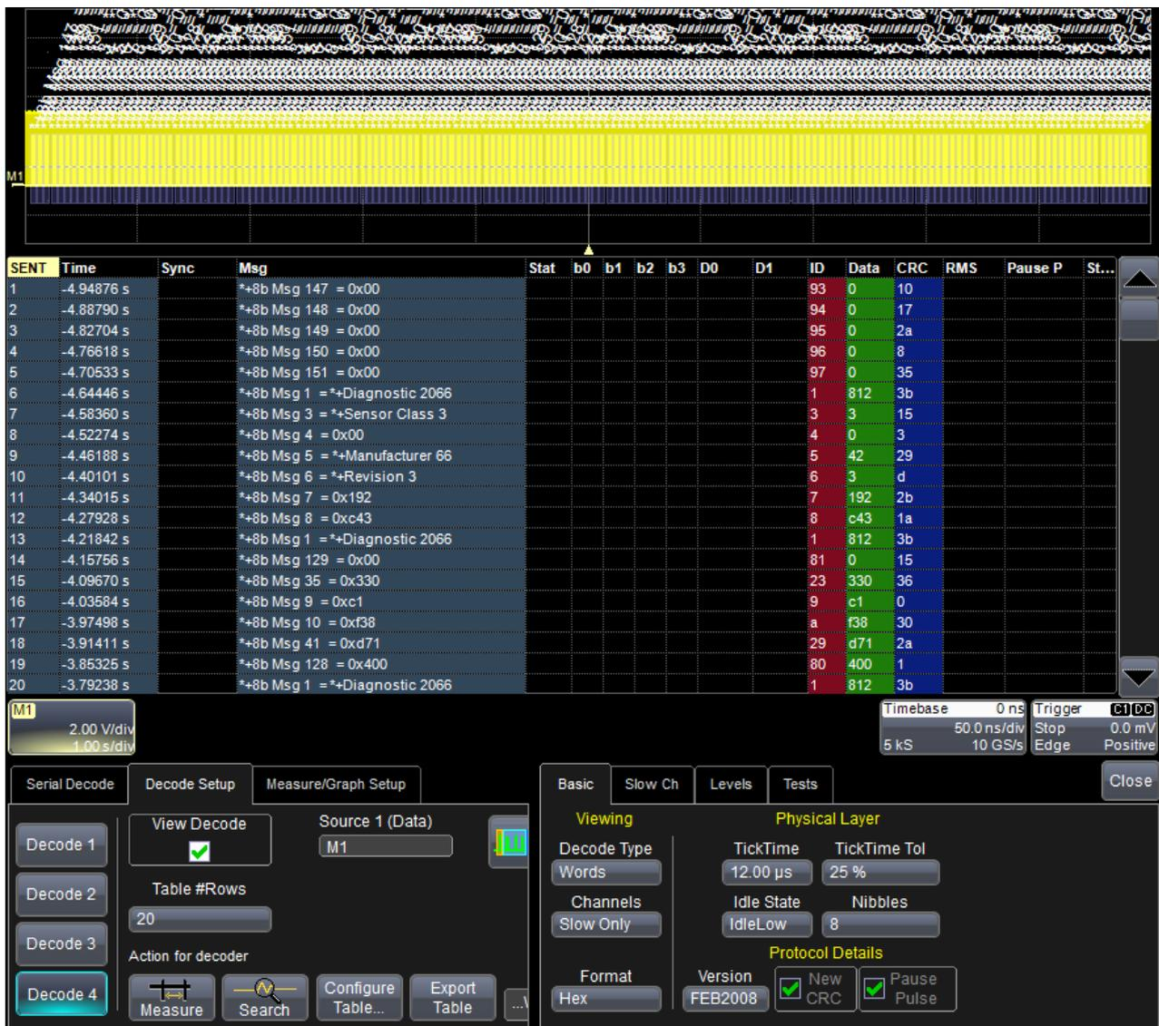
Figure 15 Slow Channel Only Decode, with slow messages IDs and Data columns, no SCDF file in use.
