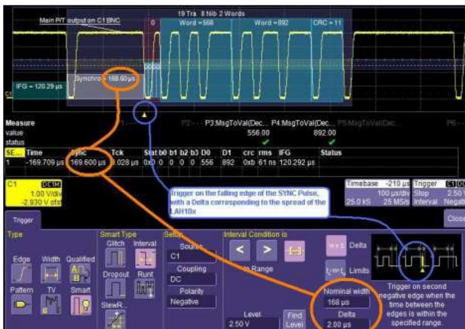
Figure 42: Setting up the Interval trigger for SENT
