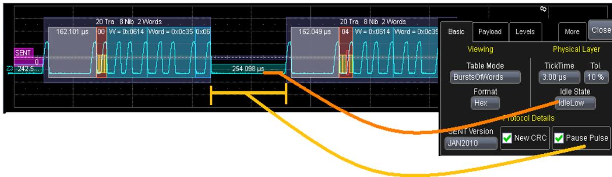
Figure 33: Example of SENT signal, 3us TickTime, Idle Low with Pause Pulse
