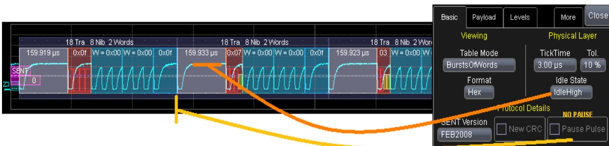
Figure 35: Example of SENT signal, 3us Tick Time, Idle High, without Pause Pulse
