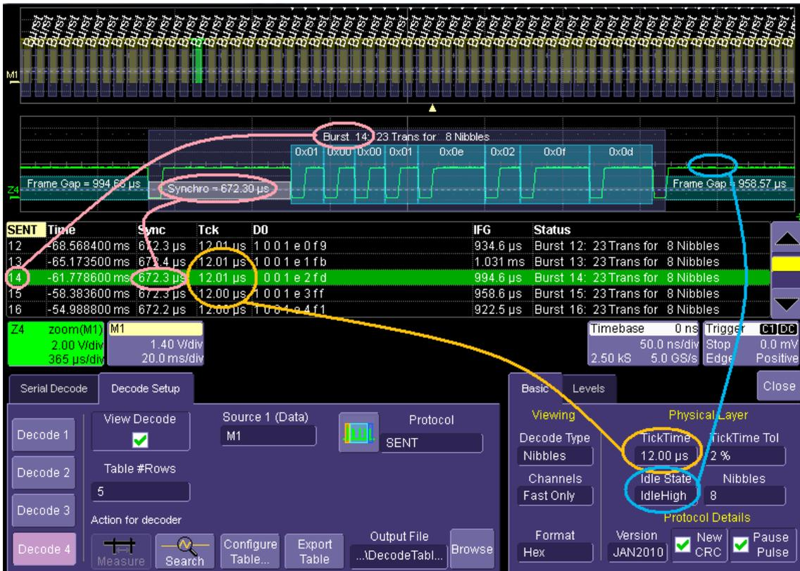
Figure 6 Example of correct Nibbles decoding with Mother Trace, Zoom and Basic Tab
