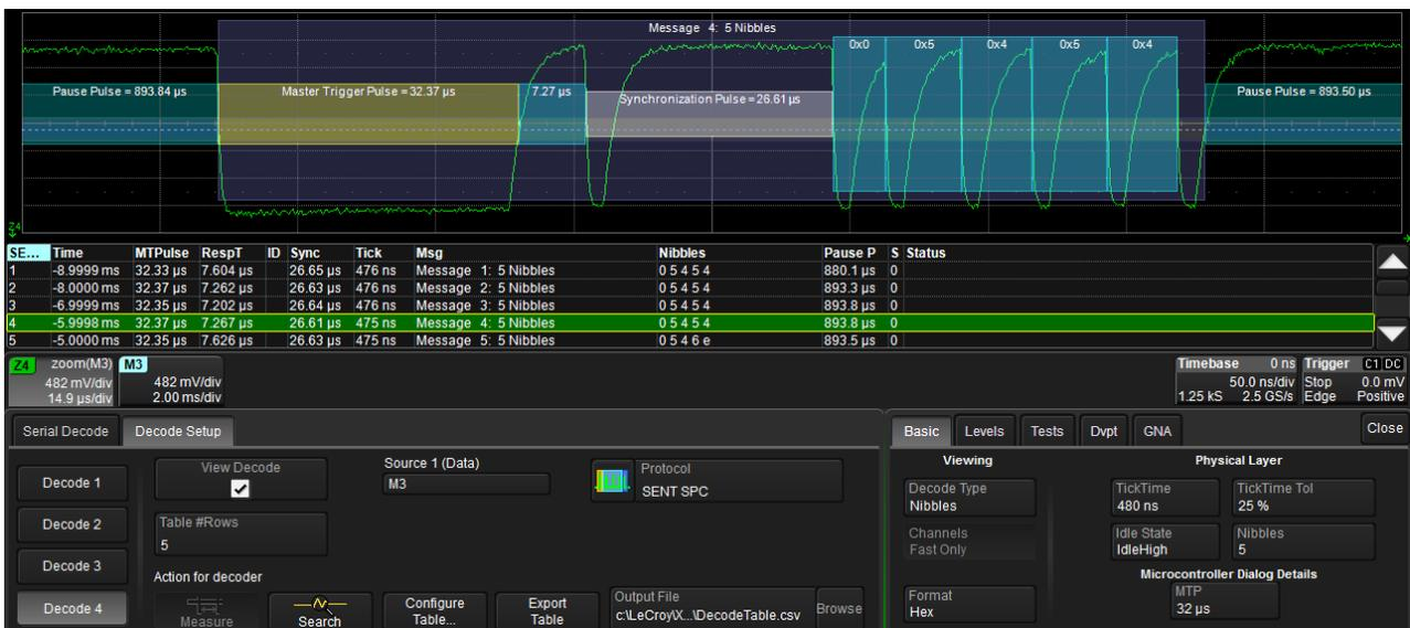
Figure 37: Example of SENT SPC signal, 480 ns Tick Time, 32 us Master Pulse, 5 Nibbles
