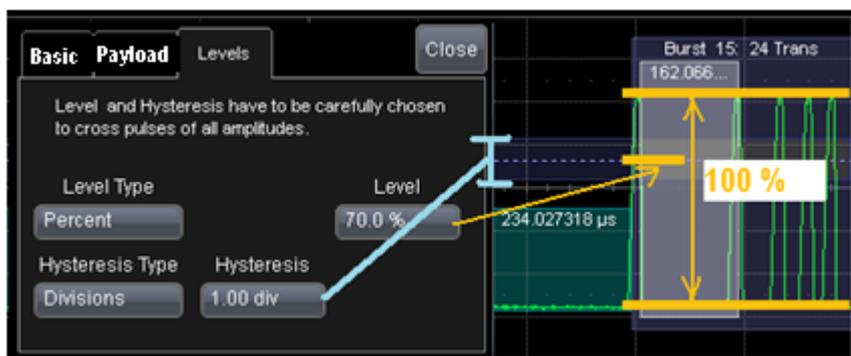
Figure 9: The Level controls and there visualization on trace
