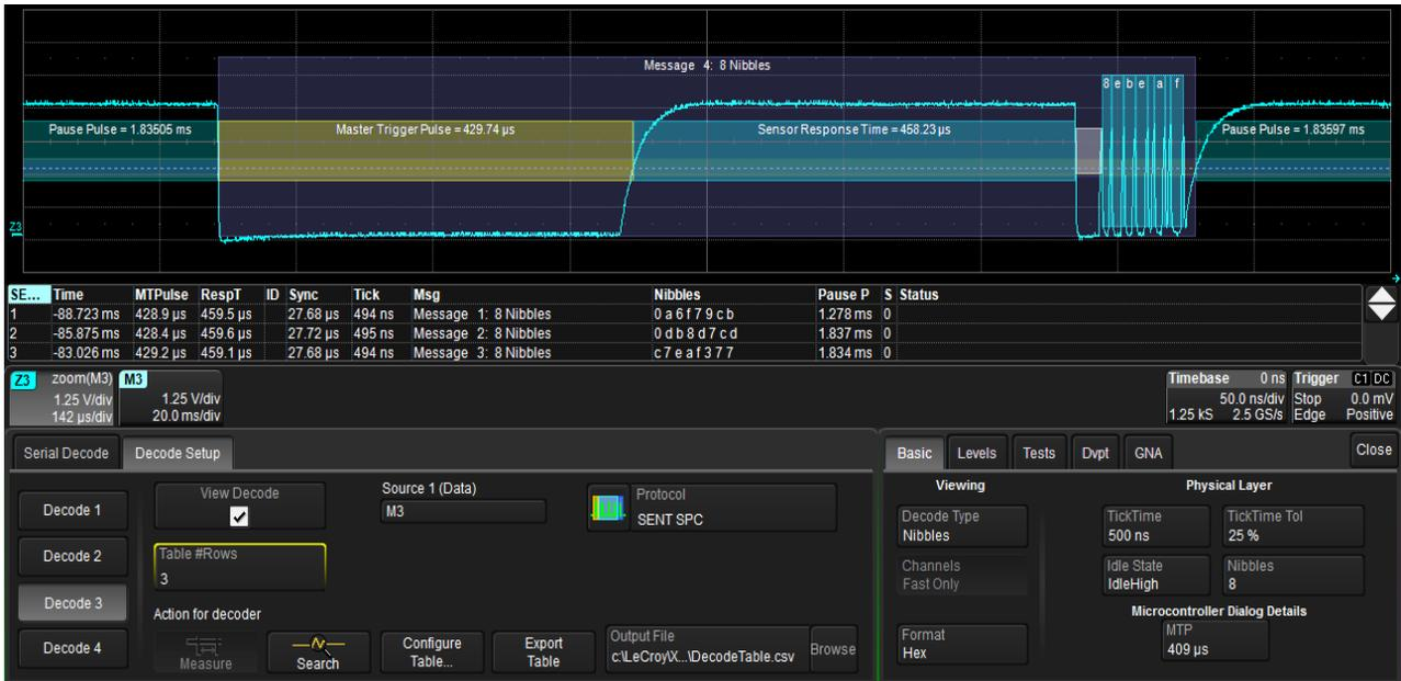
Figure 36: Example of SENT SPC signal, 500 ns Tick Time, 409 us Master Pulse, 8 Nibbles
