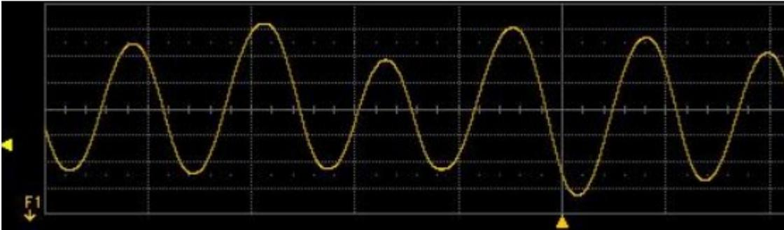
Figure 38: Typical Trend of a 12 bit Angle sensor when rotated
