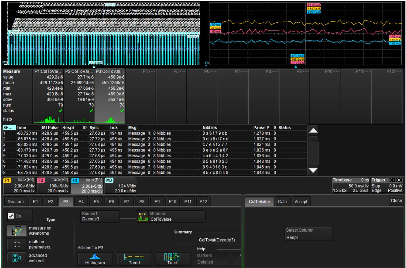
Figure 40: Graphing the MTP, the Response Time and the Pause Pulse in an SENT SPC communication
