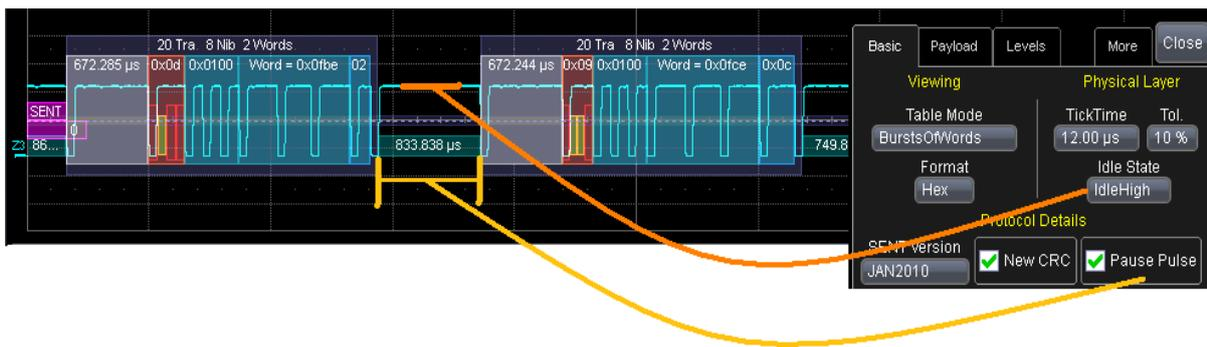
Figure 34: Example of SENT signal, 12 us TickTime, Idle high with Pause Pulse
