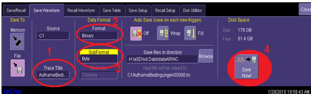
Figure 1: The Save Waveform dialog
